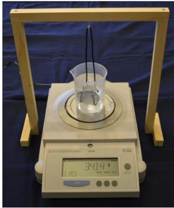
The SG apparatus above consists of a scale, a plastic container filled with water, a scaffold to suspend the coin, and a piece of plastic-coated wire bent to suspend the coin in the water without touching the sides or bottom of the beaker.
