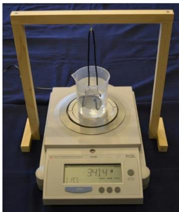
The SG apparatus above consists of a scale, a plastic container filled with water, a scaffold to suspend the coin, and a piece of plastic-coated wire bent to suspend the coin in the water without touching the sides or bottom of the beaker.
