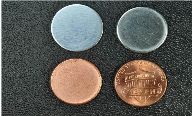
(The photo above shows a cent planchet as cut from the strip [upper left], and a similar planchet after the upsetting mill ‘upper right’. The lower photos show a copper plated planchet ready for striking and a finished 2010 cent. Planchets before upsetting are sometimes called “Type 1” and planchets after upsetting are sometimes called “Type 2.” Note how the faint lines from the rolling mill and most other planchet defects are obliterated by the pressure of the final coining.)
