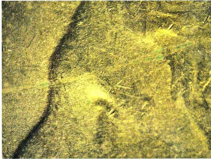
Fig 1: A streak of PVC contamination. The white part over the eye shows the surface previously under the green, which has become etched.
